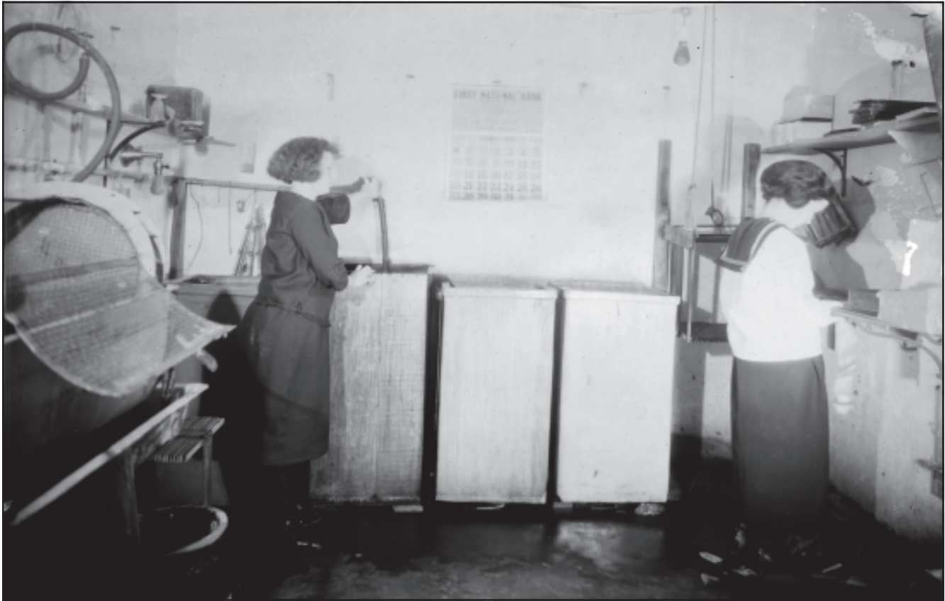
Figure 17. Dwight Church's darkroom and production facilities at Photo Park, 7 West Main Street. Unidentified assistants are at work in January, 1924. Four separate processing tanks are in the center and a drum dryer is on the left in this photo.
